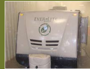
Rain Booth Testing 1/2" per minute
